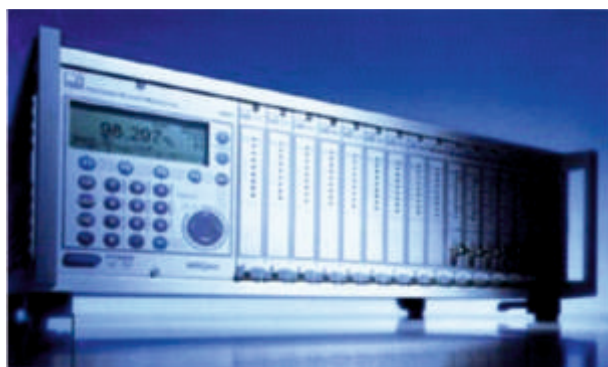
Fig. 3: A MGC plus data acquisition system
