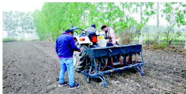
Plate 3: Field performance evaluation of prototype subsurface manure and seed applicator for sowing wheat
