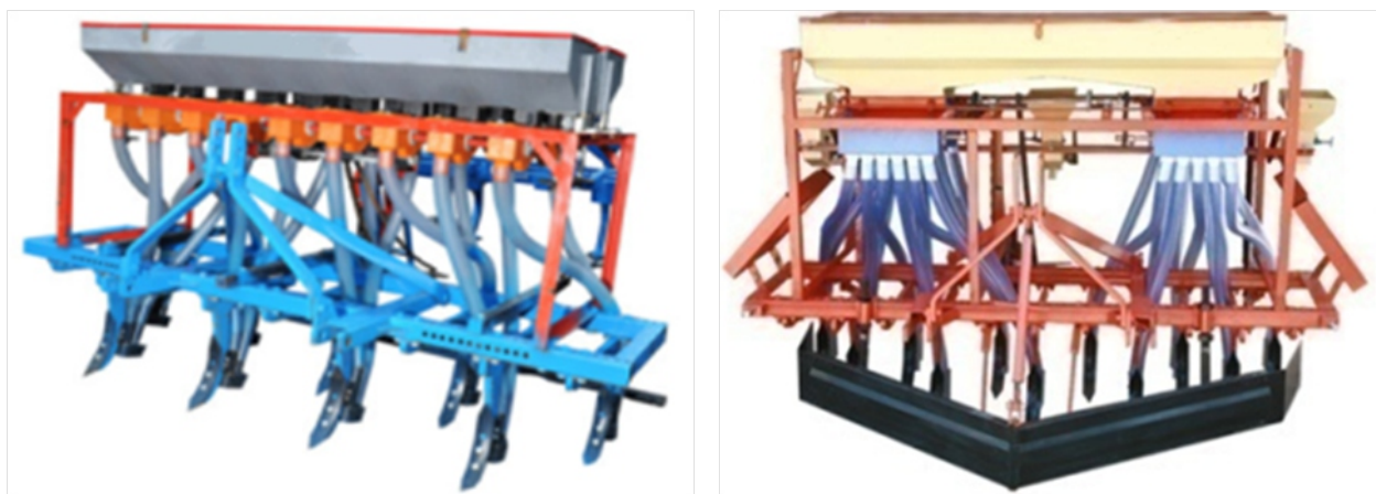
Fig. 6: Garlic seeder/planter made by Private manufacturer
