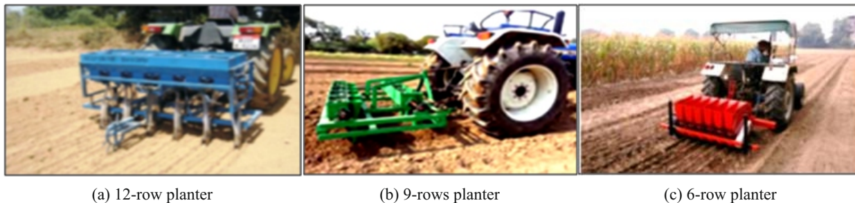
Fig. 4: Different tractor drawn garlic planter
