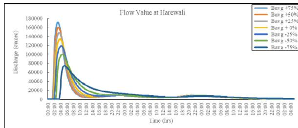
Fig. 4: Peak discharge versus time for varying breach width at Harewali
