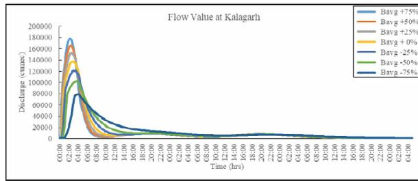
Fig. 3: Peak discharge versus time for varying breach width at Kalagarh
