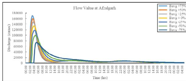
Fig. 5: Peak discharge versus time for varying breach width at Afzalgarh
