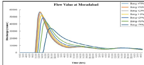
Fig. 7: Peak discharge versus time for varying breach width at Moradabad
