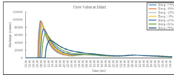
Fig. 6: Peak discharge versus time for varying breach width at Dilari
