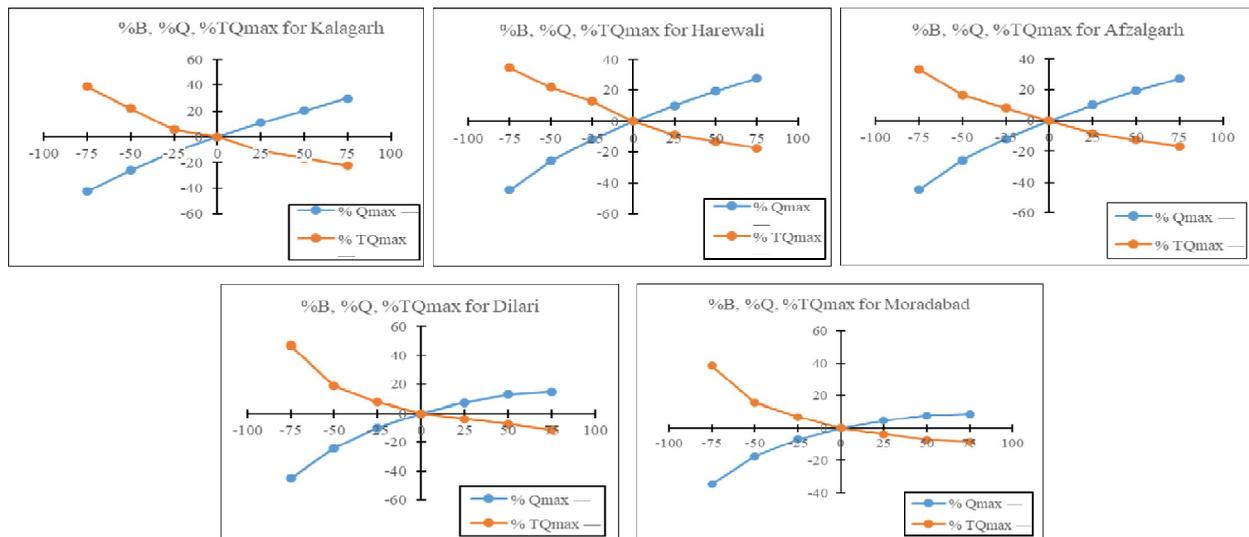
Fig. 8: Line graph between %B, %Q and % T<sub>Qmax</sub> at different five locations downstream of Ramganga dam
