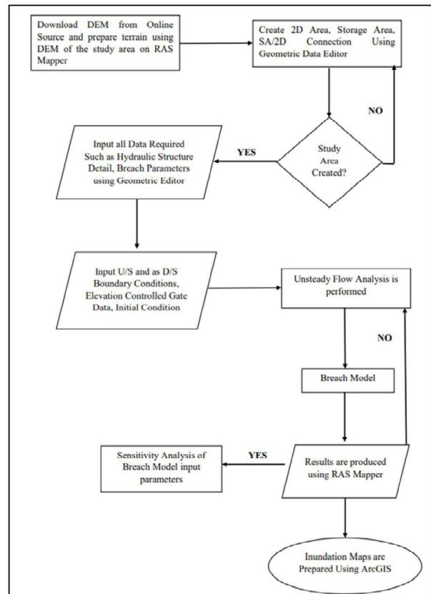
**Fig. 2: Flowchart representing 2D dam breach modelling and sensitivity analysis**
