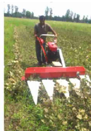
Fig. 2: Green gram crop and harvesting of green gram crop by walking type self-propelled vertical conveyor reaper-cum-windrower
