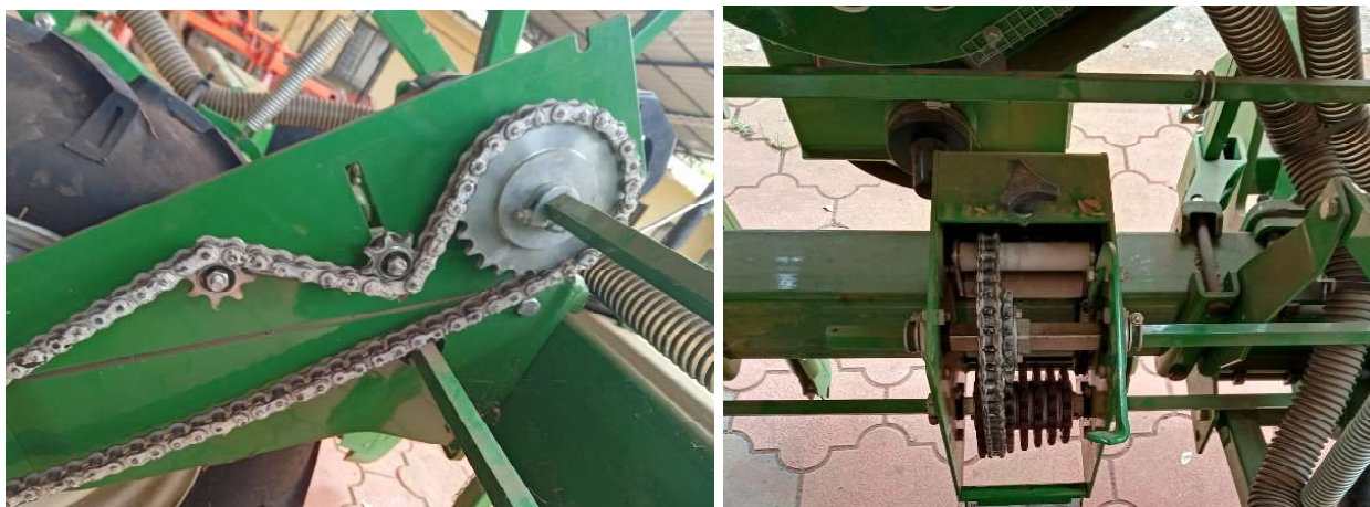
Fig 2: Transmission system of the planter to achieve different seed spacing
