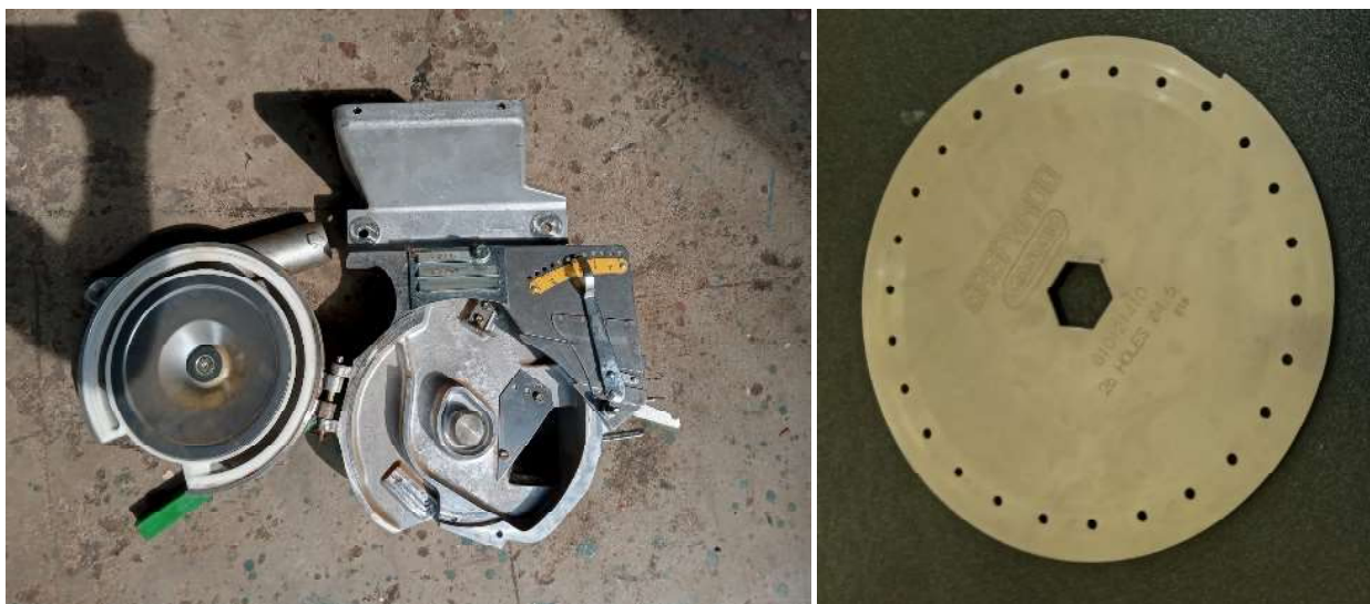
Fig. 1: Illustrates the seed metering mechanism and plate used in the planter
