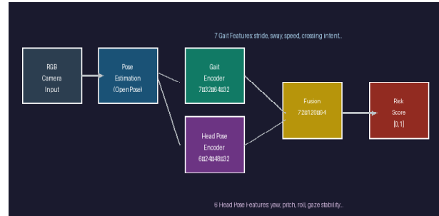
Fig. 3: Gait and Head Pose Feature Extraction Pipeline - dual-encoder behavioral signal processing
