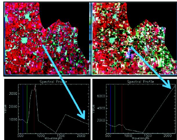
**Fig. 5: FCC images and corresponding spectral curve of pre burn and post burn pixels**
